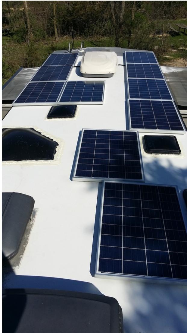
Figure 1. Standing in the middle of the roof looking rearward. Cables are routed primarily under the panels.
