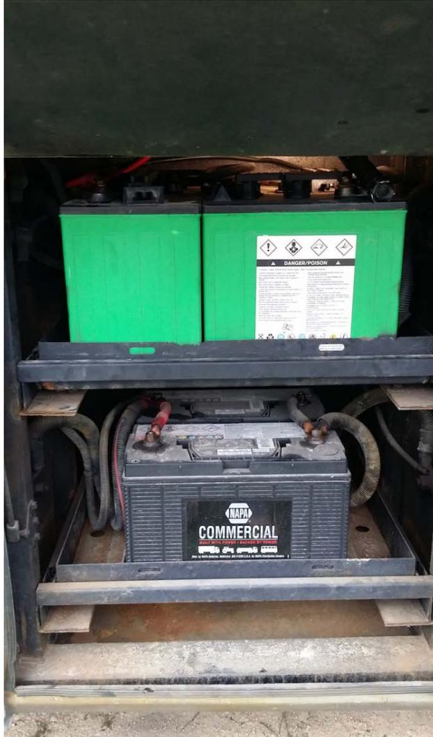
Figure 2 Four house batteries on the top slide-out tray; two chassis batteries on the bottom tray. This battery bay is located adjacent to and just forward of the bay with the controller, etc.
