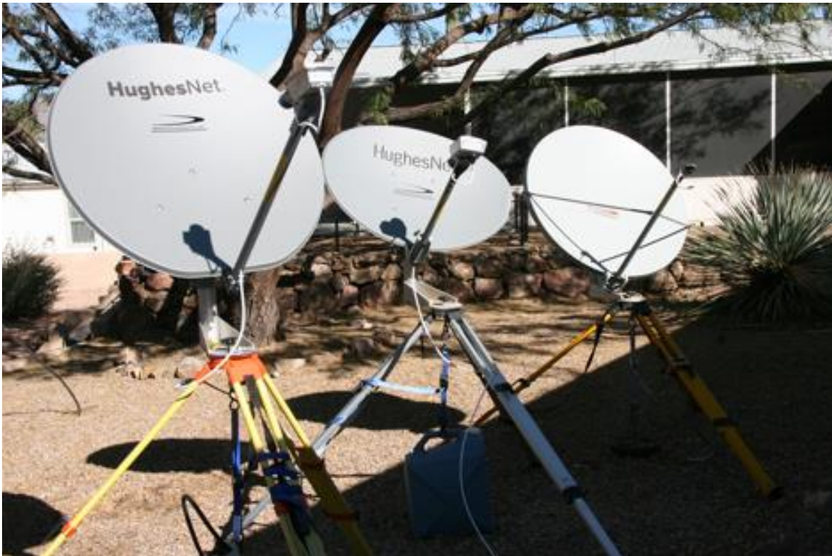
Tripod Setups – .90 m Antenna (left), .74 m Antenna (middle) & .98 m Antenna (right)
