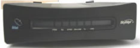
**PWR** (Power indicator): When this green LED is on, the satellite modem is powered up. This light should always be on if the system is plugged into a good power source.
