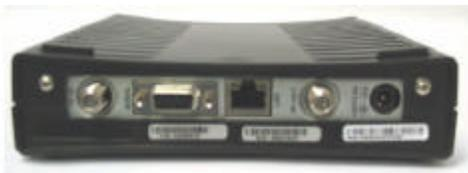
**RF-IN** (Female F-Type connector): The Rx coaxial cable from your satellite out-door unit connects to this port.
